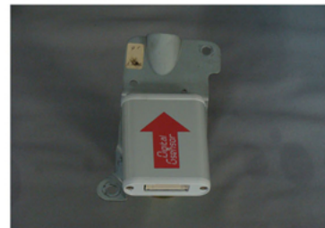
Digital G-Sensor secured to bracket
